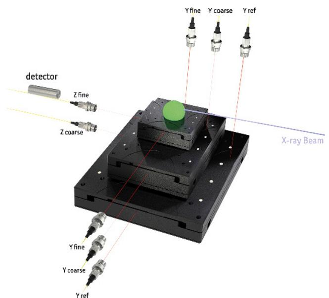
**Figure 1:** Rough sketch of the setup. The eight sensor heads M12/C1.6 are shown monitoring the 3 modules, each module consist of 3-dimensional X, Y, and Z movements. The complete setup is in high vacuum.
