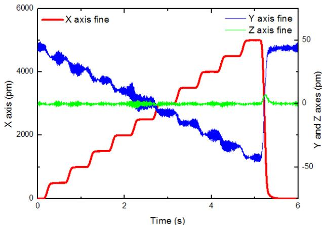
**Figure 2:** The blue curve shows the water surface and sensor head movements and the red curve represents the displacements measured on the side of the mirror after hitting the optical table with a hammer.
