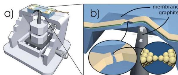
**Figure 1:** (a) Schematics of the breaking mechanism, showing the sample holder and a cut through the sample (not to scale). The image further depicts the tip, the mechanical x-y positioning stage and attocube's ANPz100 nanopositioner. (b) Zoom into panel (a), demonstrating the working principle of the setup. The typical membrane size is  $0.6 \times 0.6 \text{ mm}^2$  with a thickness of 340 nm.
