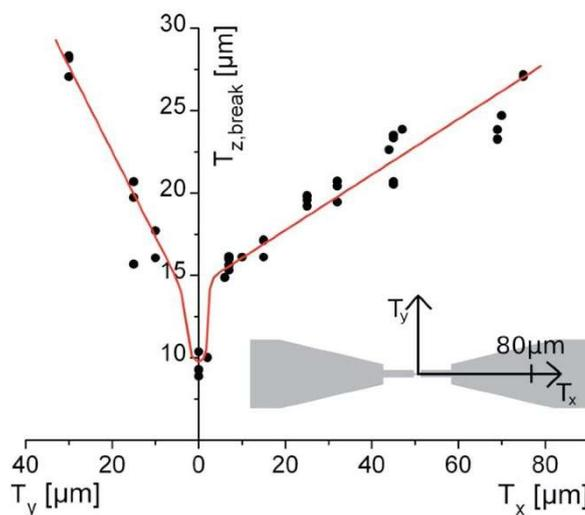
**Figure 2:** Sensitivity of the setup to lateral motion of the tip. The main panel shows the displacement in z-direction required to break a nanobridge as function of the lateral position of the tip. The directions x and y are defined in the inset.
