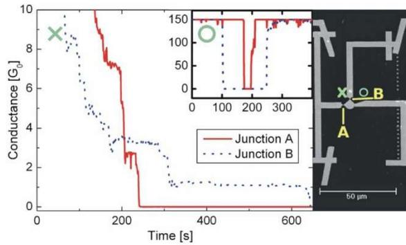
**Figure 2:** Time-dependent conductance of junctions A and B as depicted in the micrograph to the right. The tip was located at the position indicated by the green cross (the inset was recorded at the position indicated by the circle). At  $t = 160$  s the motion direction of the tip is reversed.
