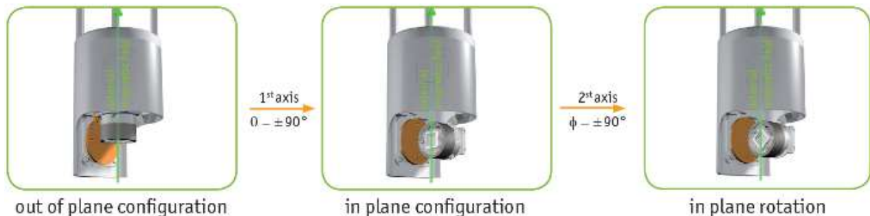
Figure 1: Working principle. The first rotation axis controls the orientation of the sample plane with respect to the fixed external magnetic field ( \theta: \pm 90^\circ ), whereas the second rotator actuates the in-plane component ( \varphi: \pm 90^\circ ). Combining both axes allows for arbitrary mutual orientations of the magnetic field vector with regards to the sample plane.
