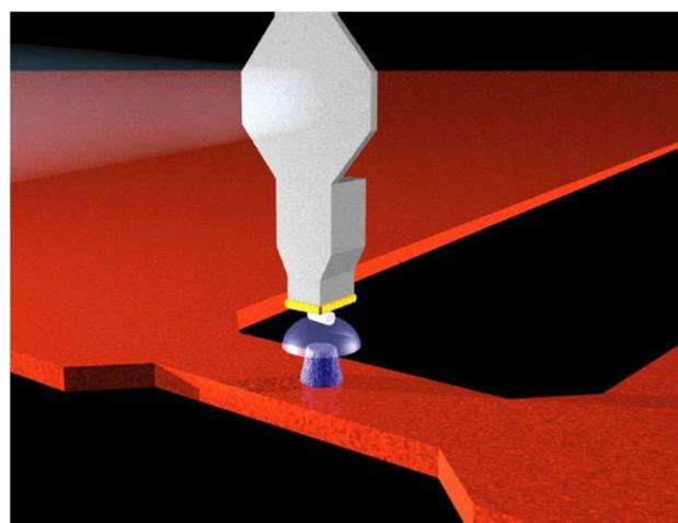
**Figure 1:** Schematic drawing of the MRFM setup showing the ultra-sensitive cantilever (grey), tobacco virus (white), and magnetic tip (blue). Magnetic resonance is achieved within the resonant slice (faint blue), where the gradient magnetic field of the tip and the rf magnetic field created by the microwire (red) satisfy the Larmor condition. The microwire and magnetic tip are brought to close proximity with the cantilever by taking advantage of two attocube ANPx51 nanopositioners.
