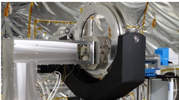
Figure 4: Calibration setup with autocollimator. Picture is provided by OHB.
