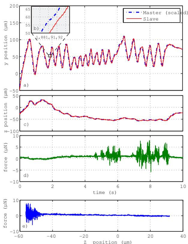
**Figure 2:** Tracking behavior and force measurement during surface approach: a) y position of oscillating gripper (slave) compared to scaled master position with b), zoomed view on position trajectory, c) z position of gripper and master, d) measured force, e) measured force over z position.
