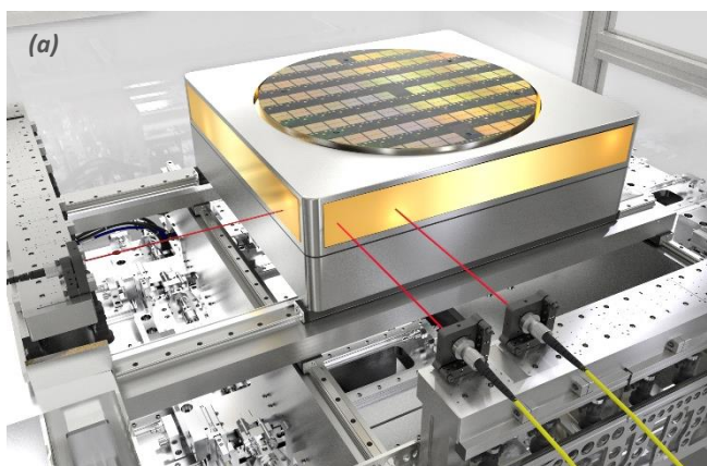
Figure 1: Two xy-stage control application examples are shown. (a) Wafer mounted on a moving stage, where mirrors are attached. Three sensor heads are fixed to the frame. The xy-movement of the stage is controlled by the IDS3010. (b) Another possible application is shown in which miniature sensor heads are mounted on the moving wafer stage, while the mirrors are fixed to the frame.
