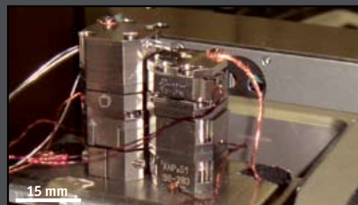
Figure 1: attocube's tuning fork based attoAFM mounted inside a LEO 1530 Scanning Electron Microscope equipped with a laser interferometry table for electron lithography (Group of Prof. Reiss, University of Bielefeld, Germany).
