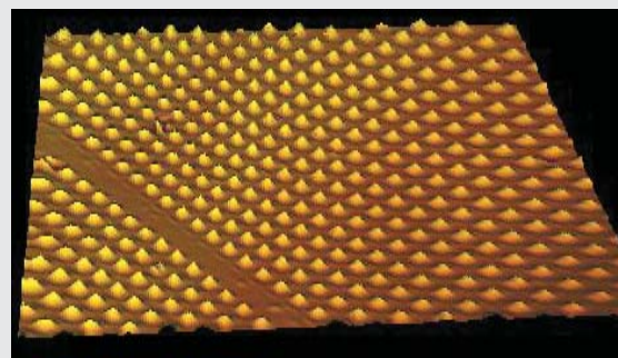
Fig. 2: Confocal picture of a chess board grating ( \text{SiO}_2 on Si) with a period of 2 microns, recorded in reflection mode. The sample has some defects on the surface structure.
