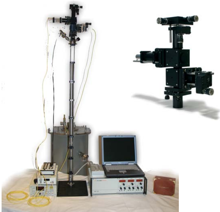
Fig. 4: Complete attoCFM system and the confocal microscope head.
