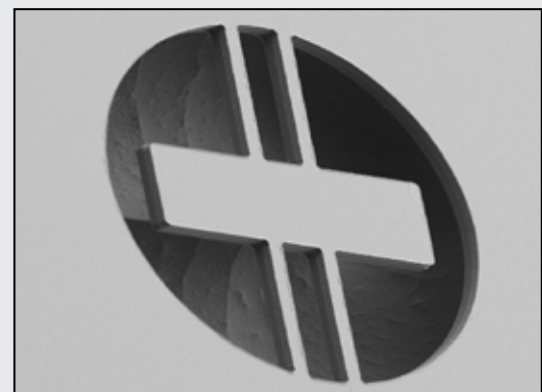
Fig. 2: Scanning electron microscope image of the optomechanical resonator, fabricated from epitaxially grown Al_xGa_{1-x}As .
